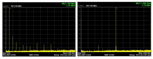
Figure 2. (Left) Measured IQ output, 100 MHz tone spectrum. (Right) Measured IQ output, 1 GHz tone spectrum.
